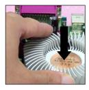
4. Press the two levers down to fasten the fan. Each lever can be pressed down in only ONE direction.
